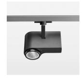
Surface-mounted luminaire with LED, rated life of the LED L80/B10 > 50000 h, colour rendering index CRI > 90, chromaticity tolerance 2 SDCM (initial), reflector with circular light distribution pattern, reflector pure aluminium 99,99% in MIRO-Silver®, segmented and faceted, exchangeable reflector unit in high-sheen black plastic, with glass cover, rotation angle 330°, swivel angle 90°, luminaire housing die-cast aluminium, powder-coated, stratoblack
