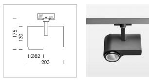
Surface-mounted luminaire with LED, rated life of the LED L80/B10 > 50000 h, chromaticity tolerance 3 SDCM (initial), reflector with circular light distribution pattern, reflector pure aluminium 99,99% in MIRO-Silver®, segmented and faceted, exchangeable reflector unit in high-sheen black plastic, with glass cover, rotation angle 330°, swivel angle 90°, luminaire housing diecast aluminium, powder-coated, stratoblack
