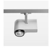
Surface-mounted luminaire with LED, rated life of the LED L80/B10 > 50000 h, colour rendering index CRI > 96, chromaticity tolerance 3 SDCM (initial), reflector with circular light distribution pattern, reflector pure aluminium 99,99% in MIRO-Silver®, segmented and faceted, exchangeable reflector unit in high-sheen black plastic, with glass cover, rotation angle 330°, swivel angle 90°, luminaire housing die-cast aluminium, powder-coated, stratosilver
