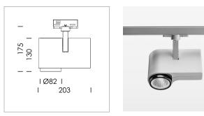
Surface-mounted luminaire with LED, rated life of the LED L80/B10 > 50000 h, chromaticity tolerance 3 SDCM (initial), reflector with circular light distribution pattern, reflector pure aluminium 99,99% in MIRO-Silver®, segmented and faceted, exchangeable reflector unit in high-sheen black plastic, with glass cover, rotation angle 330°, swivel angle 90°, luminaire housing diecast aluminium, powder-coated, stratosilver
