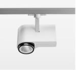
Surface-mounted luminaire with LED, rated life of the LED L80/B10 > 50000 h, chromaticity tolerance 2 SDCM (initial), reflector with circular light distribution pattern, reflector pure aluminium 99,99% in MIRO-Silver®, segmented and faceted, exchangeable reflector unit in high-sheen black plastic, with glass cover, rotation angle 330°, swivel angle 90°, luminaire housing diecast aluminium, powder-coated, stratowhite
