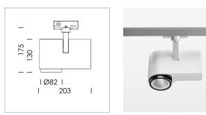
Surface-mounted luminaire with LED, rated life of the LED L80/B10 > 50000 h, chromaticity tolerance 3 SDCM (initial), reflector with circular light distribution pattern, reflector pure aluminium 99,99% in MIRO-Silver®, segmented and faceted, exchangeable reflector unit in high-sheen black plastic, with glass cover, rotation angle 330°, swivel angle 90°, luminaire housing diecast aluminium, powder-coated, stratowhite
