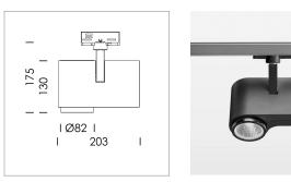
Surface-mounted luminaire with LED, rated life of the LED L80/B10 > 50000 h, colour rendering index CRI > 96, chromaticity tolerance 2 SDCM (initial), reflector with circular light distribution pattern, reflector pure aluminium 99,99% in MIRO-Silver®, segmented and faceted, exchangeable reflector unit in high-sheen black plastic, with glass cover, rotation angle 330°, swivel angle 90°, luminaire housing die-cast aluminium, powder-coated, stratoblack
