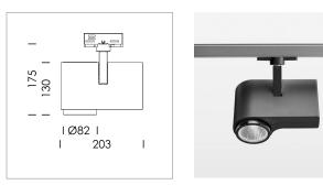
Surface-mounted luminaire with LED, rated life of the LED L80/B10 > 50000 h, chromaticity tolerance 3 SDCM (initial), reflector with circular light distribution pattern, reflector pure aluminium 99,99% in MIRO-Silver®, segmented and faceted, exchangeable reflector unit in high-sheen black plastic, with glass cover, rotation angle 330°, swivel angle 90°, luminaire housing diecast aluminium, powder-coated, stratoblack
