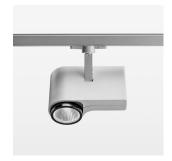
Surface-mounted luminaire with LED, rated life of the LED L80/B10 > 50000 h, colour rendering index CRI > 96, chromaticity tolerance 2 SDCM (initial), reflector with circular light distribution pattern, reflector pure aluminium 99,99% in MIRO-Silver®, segmented and faceted, exchangeable reflector unit in high-sheen black plastic, with glass cover, rotation angle 330°, swivel angle 90°, luminaire housing die-cast aluminium, powder-coated, stratosilver
