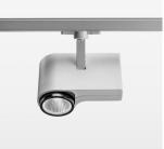
Surface-mounted luminaire with LED, rated life of the LED L80/B10 > 50000 h, chromaticity tolerance 3 SDCM (initial), reflector with circular light distribution pattern, reflector pure aluminium 99,99% in MIRO-Silver®, segmented and faceted, exchangeable reflector unit in high-sheen black plastic, with glass cover, rotation angle 330°, swivel angle 90°, luminaire housing diecast aluminium, powder-coated, stratosilver
