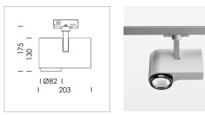
Surface-mounted luminaire with LED, rated life of the LED L80/B10 > 50000 h, chromaticity tolerance 2 SDCM (initial), LED hybrid technology, 3D silicone lens to reduce the proportion of scattered light, reflector with oval light distribution pattern, reflector pure aluminium 99,99% in MIRO-Silver®, segmented, exchangeable reflector unit in high-sheen black plastic, with glass cover, rotation angle 330°, swivel angle 90°, luminaire housing die-cast aluminium, powder-coated, stratosilver
