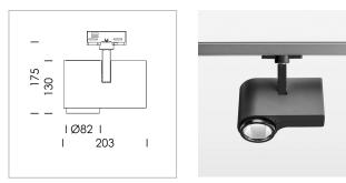
Surface-mounted luminaire with LED, rated life of the LED L80/B10 > 50000 h, chromaticity tolerance 2 SDCM (initial), LED hybrid technology, 3D silicone lens to reduce the proportion of scattered light, reflector with oval light distribution pattern, reflector pure aluminium 99,99% in MIRO-Silver®, segmented, exchangeable reflector unit in high-sheen black plastic, with glass cover, rotation angle 330°, swivel angle 90°, luminaire housing die-cast aluminium, powder-coated, stratoblack
