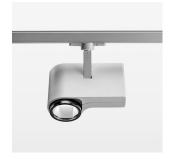
Surface-mounted luminaire with LED, rated life of the LED L80/B10 > 50000 h, chromaticity tolerance 3 SDCM (initial), LED hybrid technology, 3D silicone lens to reduce the proportion of scattered light, reflector with oval light distribution pattern, reflector pure aluminium 99,99% in MIRO-Silver®, segmented, exchangeable reflector unit in high-sheen black plastic, with glass cover, rotation angle 330°, swivel angle 90°, luminaire housing die-cast aluminium, powder-coated, stratosilver
