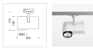
Surface-mounted luminaire with LED, rated life of the LED L80/B10 > 50000 h, chromaticity tolerance 3 SDCM (initial), LED hybrid technology, 3D silicone lens to reduce the proportion of scattered light, reflector with oval light distribution pattern, reflector pure aluminium 99,99% in MIRO-Silver®, segmented, exchangeable reflector unit in high-sheen black plastic, with glass cover, rotation angle 330°, swivel angle 90°, luminaire housing die-cast aluminium, powder-coated, stratowhite
