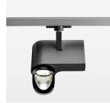
Surface-mounted luminaire with LED, rated life of the LED L80/B10 > 50000 h, chromaticity tolerance 2 SDCM (initial), reflector with asymmetrical light distribution pattern, primary reflector and kick reflector 99% pure aluminium in MIRO-Silver®, attachment with kick reflector to the ceiling approach of the light cone, exchangeable reflector unit in high-sheen black plastic, with glass cover, rotation angle 330°, swivel angle 90°, luminaire housing die-cast aluminium, powder-coated, stratoblack
