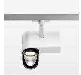
Surface-mounted luminaire with LED, rated life of the LED L80/B10 > 50000 h, chromaticity tolerance 2 SDCM (initial), reflector with asymmetrical light distribution pattern, primary reflector and kick reflector 99% pure aluminium in MIRO-Silver®, attachment with kick reflector to the ceiling approach of the light cone, exchangeable reflector unit in high-sheen black plastic, with glass cover, rotation angle 330°, swivel angle 90°, luminaire housing die-cast aluminium, powder-coated, stratowhite
