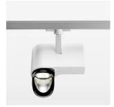
Surface-mounted luminaire with LED, rated life of the LED L80/B10 > 50000 h, chromaticity tolerance 3 SDCM (initial), reflector with asymmetrical light distribution pattern, primary reflector and kick reflector 99% pure aluminium in MIRO-Silver®, attachment with kick reflector to the ceiling approach of the light cone, exchangeable reflector unit in high-sheen black plastic, with glass cover, rotation angle 330°, swivel angle 90°, luminaire housing die-cast aluminium, powder-coated, stratowhite
