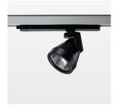
Surface-mounted luminaire with LED, rated life of the LED L80/B10 > 50000 h, colour rendering index CRI > 80, chromaticity tolerance 2 SDCM (initial), reflector with circular light distribution pattern, reflector pure aluminium 99,99% in MIRO-Silver®, rotation angle 330°, swivel angle +85°/-85°, luminaire head/retention arm die-cast aluminium, powder-coated, stratoblack
