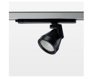
Surface-mounted luminaire with LED, rated life of the LED L80/B10 > 50000 h, colour rendering index CRI > 90, chromaticity tolerance 2 SDCM (initial), reflector with circular light distribution pattern, reflector pure aluminium 99,99% in MIRO-Silver®, rotation angle 330°, swivel angle +85°/-85°, luminaire head/retention arm die-cast aluminium, powder-coated, stratoblack
