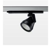
Surface-mounted luminaire with LED, rated life of the LED L80/B10 > 50000 h, colour rendering index CRI > 96, chromaticity tolerance 3 SDCM (initial), reflector with circular light distribution pattern, reflector pure aluminium 99,99% in MIRO-Silver®, rotation angle 330°, swivel angle +85°/-85°, luminaire head/retention arm die-cast aluminium, powder-coated, stratoblack
