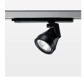
Surface-mounted luminaire with LED, rated life of the LED L80/B10 > 50000 h, colour rendering index CRI > 90, chromaticity tolerance 2 SDCM (initial), reflector with oval light distribution pattern, reflector pure aluminium 99,99% in MIRO-Silver®, rotation angle 330°, swivel angle +85°/-85°, luminaire head/retention arm die-cast aluminium, powder-coated, stratoblack
