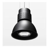
Suspended luminaire with LED, rated life of the LED L80/B10 > 50000 h, chromaticity tolerance 3 SDCM (initial), reflector with circular light distribution pattern, reflector pure aluminium 99,99% in MIRO-Silver®, luminaire shade die-cast aluminium, powder-coated, swivel angle +25°/-25°, luminaire housing sheet steel, powder-coated, stratoblack
