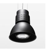
Suspended luminaire with LED, rated life of the LED L80/B10 > 50000 h, chromaticity tolerance 3 SDCM (initial), reflector with circular light distribution pattern, reflector pure aluminium 99,99% in MIRO-Silver®, luminaire shade die-cast aluminium, powder-coated, swivel angle +25°/-25°, luminaire housing sheet steel, powder-coated, stratoblack
