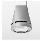
Suspended luminaire with LED, rated life of the LED L80/B10 > 50000 h, chromaticity tolerance 3 SDCM (initial), reflector with circular light distribution pattern, reflector pure aluminium 99,99% in MIRO-Silver®, luminaire head die-cast aluminium, powder-coated, stratosilver
