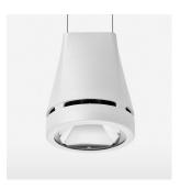
Suspended luminaire with LED, rated life of the LED L80/B10 > 50000 h, chromaticity tolerance 2 SDCM (initial), reflector with circular light distribution pattern, reflector pure aluminium 99,99% in MIRO-Silver®, luminaire head die-cast aluminium, powder-coated, stratowhite
