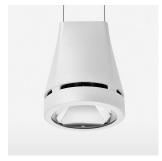
Suspended luminaire with LED, rated life of the LED L80/B10 > 50000 h, chromaticity tolerance 2 SDCM (initial), reflector with circular light distribution pattern, reflector pure aluminium 99,99% in MIRO-Silver®, luminaire head die-cast aluminium, powder-coated, stratowhite
