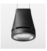
Suspended luminaire with LED, rated life of the LED L80/B10 > 50000 h, colour rendering index CRI > 80, chromaticity tolerance 2 SDCM (initial), reflector with oval light distribution pattern, reflector pure aluminium 99,99% in MIRO-Silver®, luminaire head die-cast aluminium, powder-coated, stratoblack
