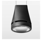
Suspended luminaire with LED, rated life of the LED L80/B10 > 50000 h, colour rendering index CRI > 80, chromaticity tolerance 2 SDCM (initial), reflector with oval light distribution pattern, reflector pure aluminium 99,99% in MIRO-Silver®, luminaire head die-cast aluminium, powder-coated, stratoblack
