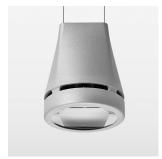
Suspended luminaire with LED, rated life of the LED L80/B10 > 50000 h, colour rendering index CRI > 80, chromaticity tolerance 2 SDCM (initial), reflector with oval light distribution pattern, reflector pure aluminium 99,99% in MIRO-Silver®, luminaire head die-cast aluminium, powder-coated, stratosilver
