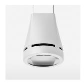
Suspended luminaire with LED, rated life of the LED L80/B10 > 50000 h, colour rendering index CRI > 90, chromaticity tolerance 2 SDCM (initial), reflector with oval light distribution pattern, reflector pure aluminium 99,99% in MIRO-Silver®, luminaire head die-cast aluminium, powder-coated, stratowhite
