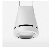
Suspended luminaire with LED, rated life of the LED L80/B10 > 50000 h, chromaticity tolerance 2 SDCM (initial), reflector with oval light distribution pattern, reflector pure aluminium 99,99% in MIRO-Silver®, luminaire head die-cast aluminium, powder-coated, stratowhite
