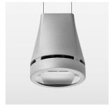
Suspended luminaire with LED, rated life of the LED L80/B10 > 50000 h, colour rendering index CRI > 90, chromaticity tolerance 2 SDCM (initial), reflector with oval light distribution pattern, reflector pure aluminium 99,99% in MIRO-Silver®, luminaire head die-cast aluminium, powder-coated, stratosilver
