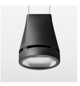
Suspended luminaire with LED, rated life of the LED L80/B10 > 50000 h, colour rendering index CRI > 80, chromaticity tolerance 2 SDCM (initial), reflector with oval light distribution pattern, reflector pure aluminium 99,99% in MIRO-Silver®, luminaire head die-cast aluminium, powder-coated, stratoblack
