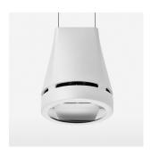
Suspended luminaire with LED, rated life of the LED L80/B10 > 50000 h, colour rendering index CRI > 90, chromaticity tolerance 2 SDCM (initial), reflector with oval light distribution pattern, reflector pure aluminium 99,99% in MIRO-Silver®, luminaire head die-cast aluminium, powder-coated, stratowhite
