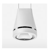
Suspended luminaire with LED, rated life of the LED L80/B10 > 50000 h, colour rendering index CRI > 80, chromaticity tolerance 2 SDCM (initial), reflector with circular light distribution pattern, reflector pure aluminium 99,99% in MIRO-Silver®, luminaire head die-cast aluminium, powder-coated, stratowhite
