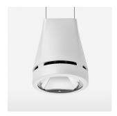
Suspended luminaire with LED, rated life of the LED L80/B10 > 50000 h, colour rendering index CRI > 90, chromaticity tolerance 2 SDCM (initial), reflector with circular light distribution pattern, reflector pure aluminium 99,99% in MIRO-Silver®, luminaire head die-cast aluminium, powder-coated, stratowhite
