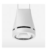
Suspended luminaire with LED, rated life of the LED L80/B10 > 50000 h, chromaticity tolerance 3 SDCM (initial), reflector with circular light distribution pattern, reflector pure aluminium 99,99% in MIRO-Silver®, luminaire head die-cast aluminium, powder-coated, stratowhite
