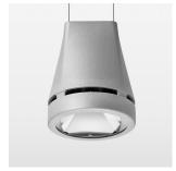
Suspended luminaire with LED, rated life of the LED L80/B10 > 50000 h, chromaticity tolerance 3 SDCM (initial), reflector with circular light distribution pattern, reflector pure aluminium 99,99% in MIRO-Silver®, luminaire head die-cast aluminium, powder-coated, stratosilver
