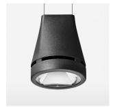
Suspended luminaire with LED, rated life of the LED L80/B10 > 50000 h, colour rendering index CRI > 90, chromaticity tolerance 2 SDCM (initial), reflector with circular light distribution pattern, reflector pure aluminium 99,99% in MIRO-Silver®, canopy sheet steel, powder-coated, luminaire head die-cast aluminium, powder-coated, stratoblack
