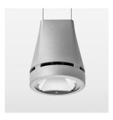
Suspended luminaire with LED, rated life of the LED L80/B10 > 50000 h, chromaticity tolerance 3 SDCM (initial), reflector with circular light distribution pattern, reflector pure aluminium 99,99% in MIRO-Silver®, canopy sheet steel, powder-coated, luminaire head die-cast aluminium, powder-coated, stratosilver
