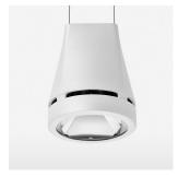
Suspended luminaire with LED, rated life of the LED L80/B10 > 50000 h, colour rendering index CRI > 90, chromaticity tolerance 2 SDCM (initial), reflector with circular light distribution pattern, reflector pure aluminium 99,99% in MIRO-Silver®, canopy sheet steel, powder-coated, luminaire head die-cast aluminium, powder-coated, stratowhite
