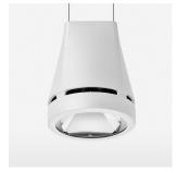
Suspended luminaire with LED, rated life of the LED L80/B10 > 50000 h, chromaticity tolerance 3 SDCM (initial), reflector with circular light distribution pattern, reflector pure aluminium 99,99% in MIRO-Silver®, canopy sheet steel, powder-coated, luminaire head die-cast aluminium, powder-coated, stratowhite
