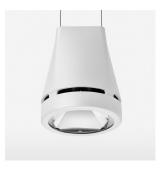
Suspended luminaire with LED, rated life of the LED L80/B10 > 50000 h, colour rendering index CRI > 90, chromaticity tolerance 2 SDCM (initial), reflector with circular light distribution pattern, reflector pure aluminium 99,99% in MIRO-Silver®, canopy sheet steel, powder-coated, luminaire head die-cast aluminium, powder-coated, stratowhite
