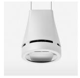
Suspended luminaire with LED, rated life of the LED L80/B10 > 50000 h, chromaticity tolerance 3 SDCM (initial), reflector with oval light distribution pattern, reflector pure aluminium 99,99% in MIRO-Silver®, canopy sheet steel, powder-coated, luminaire head die-cast aluminium, powder-coated, stratowhite
