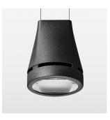
Suspended luminaire with LED, rated life of the LED L80/B10 > 50000 h, chromaticity tolerance 2 SDCM (initial), reflector with oval light distribution pattern, reflector pure aluminium 99,99% in MIRO-Silver®, canopy sheet steel, powder-coated, luminaire head die-cast aluminium, powder-coated, stratoblack
