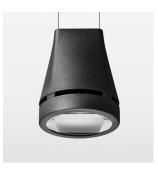
Suspended luminaire with LED, rated life of the LED L80/B10 > 50000 h, chromaticity tolerance 3 SDCM (initial), reflector with oval light distribution pattern, reflector pure aluminium 99,99% in MIRO-Silver®, canopy sheet steel, powder-coated, luminaire head die-cast aluminium, powder-coated, stratoblack
