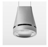
Suspended luminaire with LED, rated life of the LED L80/B10 > 50000 h, chromaticity tolerance 3 SDCM (initial), reflector with oval light distribution pattern, reflector pure aluminium 99,99% in MIRO-Silver®, canopy sheet steel, powder-coated, luminaire head die-cast aluminium, powder-coated, stratosilver
