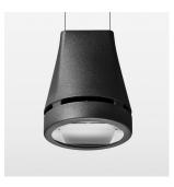
Suspended luminaire with LED, rated life of the LED L80/B10 > 50000 h, chromaticity tolerance 2 SDCM (initial), reflector with oval light distribution pattern, reflector pure aluminium 99,99% in MIRO-Silver®, canopy sheet steel, powder-coated, luminaire head die-cast aluminium, powder-coated, stratoblack
