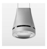
Suspended luminaire with LED, rated life of the LED L80/B10 > 50000 h, colour rendering index CRI > 90, chromaticity tolerance 2 SDCM (initial), reflector with oval light distribution pattern, reflector pure aluminium 99,99% in MIRO-Silver®, canopy sheet steel, powder-coated, luminaire head die-cast aluminium, powder-coated, stratosilver
