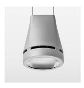
Suspended luminaire with LED, rated life of the LED L80/B10 > 50000 h, chromaticity tolerance 3 SDCM (initial), reflector with oval light distribution pattern, reflector pure aluminium 99,99% in MIRO-Silver®, canopy sheet steel, powder-coated, luminaire head die-cast aluminium, powder-coated, stratosilver
